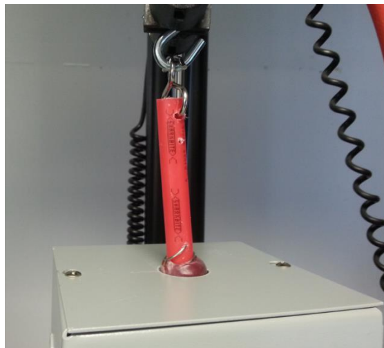
FIGURE 12- Tensile pull testing set up
